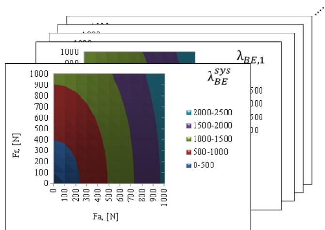
(1) Distribution diagram of failure rate ( $\lambda_{BE}^{sys}$  and  $\lambda_{BE,i}$ )
