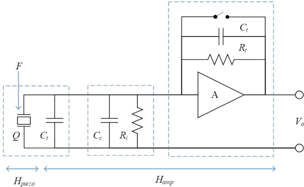
**Fig. 12** Simplified circuit diagram of charge amplifier with piezoelectric sensor
