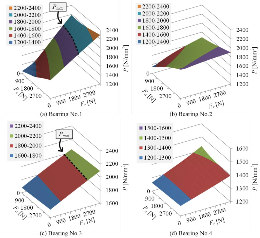
**Fig. 9** Distribution diagram of bearing surface pressure
