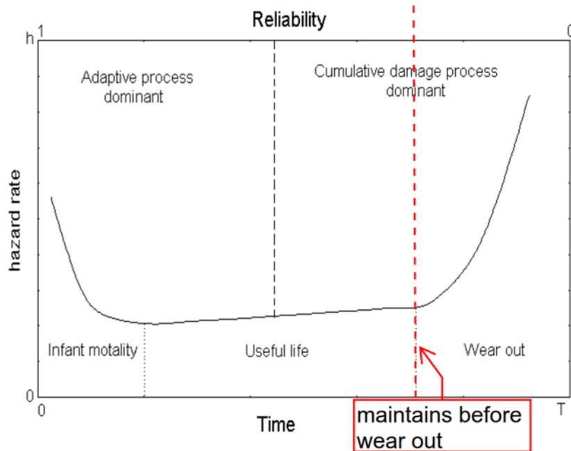
**Fig. 2** Hazard rate bathtub curve
