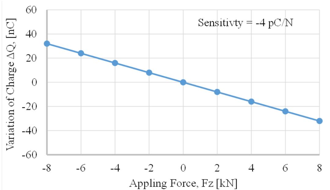
**Fig. 13** Characteristics of piezoelectric force sensor, an example for sensitivity of -4 pC/N
