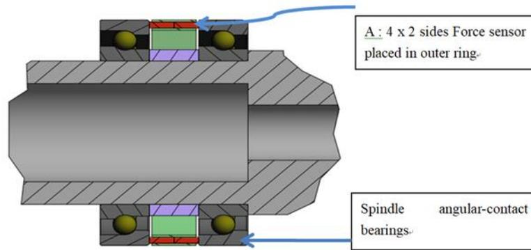
Fig. 10 Spindle bearings with force sensor assembly
