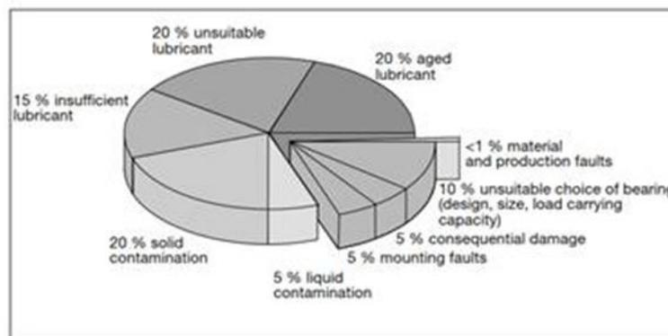
Fig 3 Bearing failure analysis (Info: FAG)
