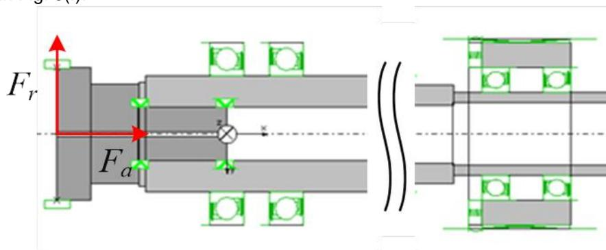
**Fig. 6** Bearing arrangements of motorized spindle (not to scale)
