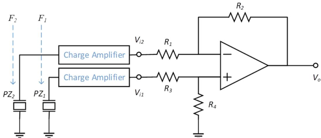
**Fig. 16** Differential amplifier as second stage
