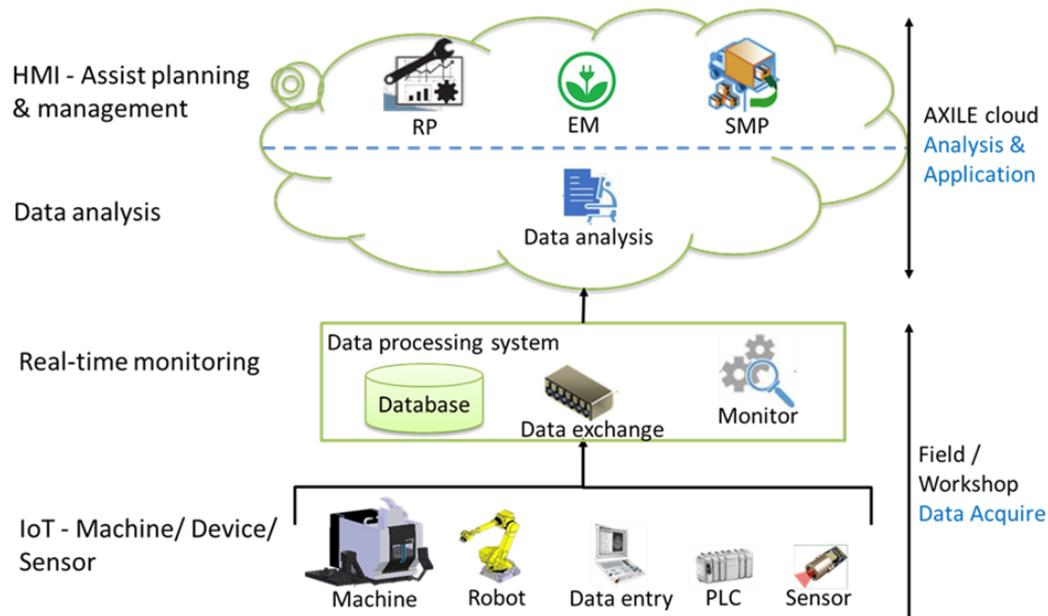
**Fig. 1** Four Layers Design
