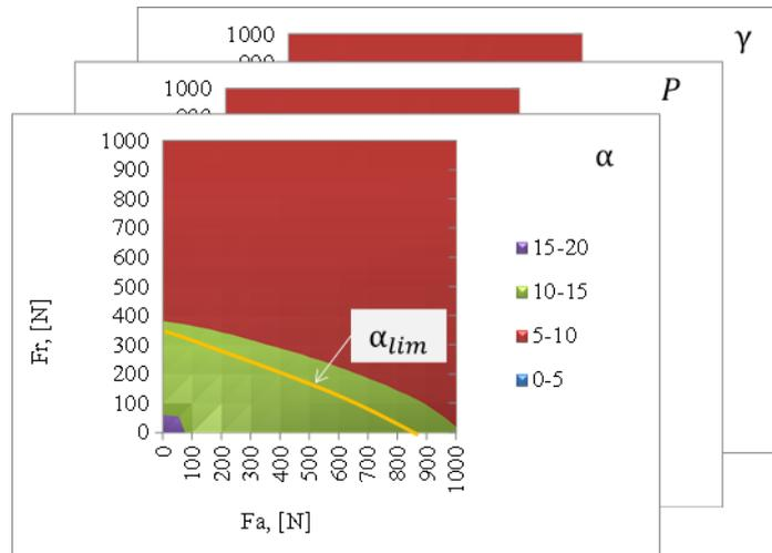
(2) Distribution diagram of contact angle, contact press, and spin-roll ratio
