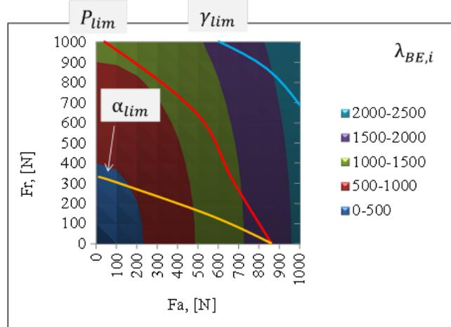
Fig. 5 Diagram of working area for a single bearing
