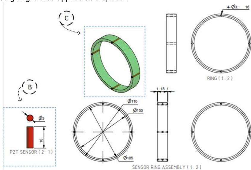
Fig. 11 Holding ring and sensor
