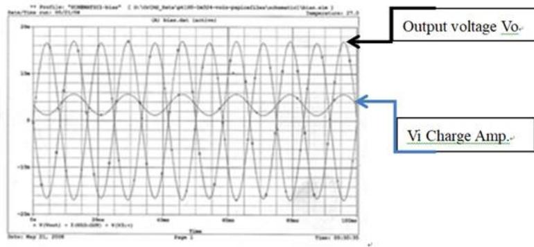
Fig. 17 Simulation of differential amplifier
